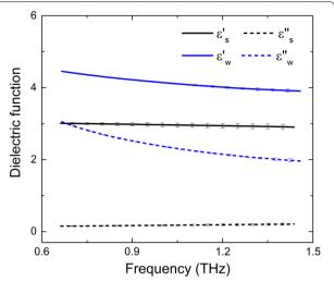
**Fig. 3** The real ( $\epsilon'$ ) and imaginary ( $\epsilon''$ ) parts of the dielectric functions of solid matter ( $\epsilon_s$ , black lines) and water ( $\epsilon_w$ , blue lines) measured by THz-TDS and THz-ATR, respectively
