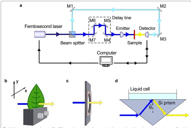
**Fig. 2** Schematic diagrams of a typical THz-TDS setup (**a**), and sketch of supporting holders, including XY two dimensional moving stage (**b**), solid sample cell (**c**) and ATR geometry (**d**)
