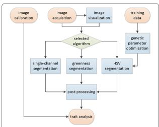
**Fig. 1** Flowchart of implemented processes: the main process (both on-the-fly and batch mode) start with the *image acquisition* as input and ends with analyzed traits. *Image calibration* allows to convert pixel metric into real-world values. Additionally, *training data* can be used to optimize parameters for HSV segmentation
