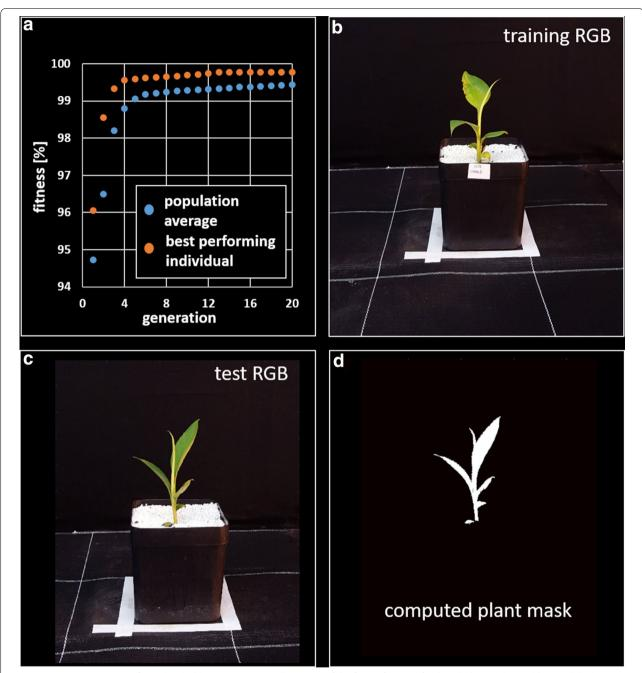
**Fig. 3** Genetic optimization of HSV thresholding parameters: **a** Illustration of the fitness function for the whole population (blue) and the best performing individual (red); after 3 generations more than 99% of the pixels are classified correctly (99.75% after 12 generations). **b** Training image, which served as the input for the optimization process; **c** test image and **d** corresponding test image mask that was computed with the optimized HSV parameter set
