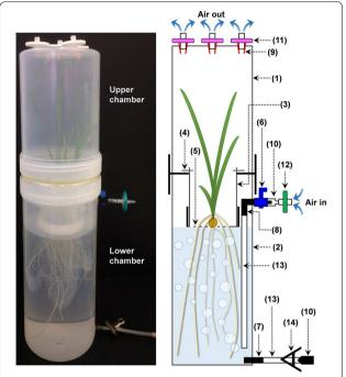
**Fig. 1** A photograph and a schematic drawing of the hydroponic system. The system is mainly comprised of an upper chamber that contains aerial part of the plant and a lower chamber that contains the nutrient solution and the plant root system. The plant is held between the two compartments with a plant holder insert. Numbers in bracket represent the part numbers listed in Table 2
