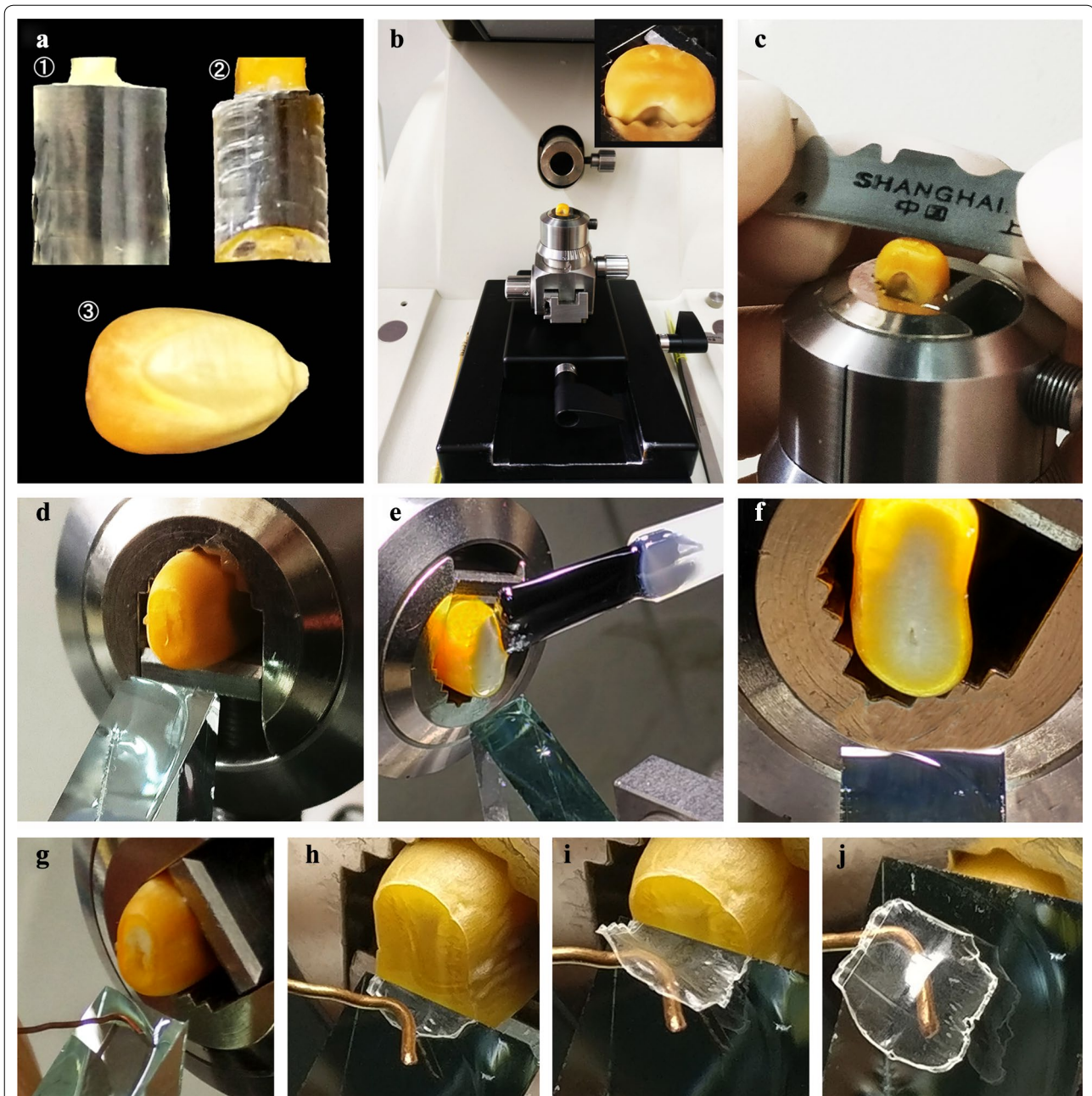
Fig. 2 The preparing method of whole section of starchy seed. a, b the small seeds and the pieces of large seeds were glued to resin blocks ( a-① , a-② ), and the resin blocks and some large seeds ( a-③ ) were clamped in the trimmer ( a ). c Sample surface was trimmed using a razor blade. d The surface was polished by a glass knife. e For floury seeds, the polished surface of sample was covered with transparent nail polish. f The excess nail polish was removed from sample surface using glass knife after nail polish solidification. g The hook was put near the blade edge before cutting. h, i A semithin section of 2 \mu\text{m} thickness was sectioned with the hook preventing section curling up or down. j The section was transferred to the slide with the hook
