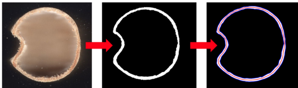
Fig. 4 Three steps of the image segmentation process. We first imported an image to MATLAB (left), then we separated the rind pixels from the pith pixels using the segmenter tool (middle), then relevant quantities were calculated using MATLAB functions (right)
