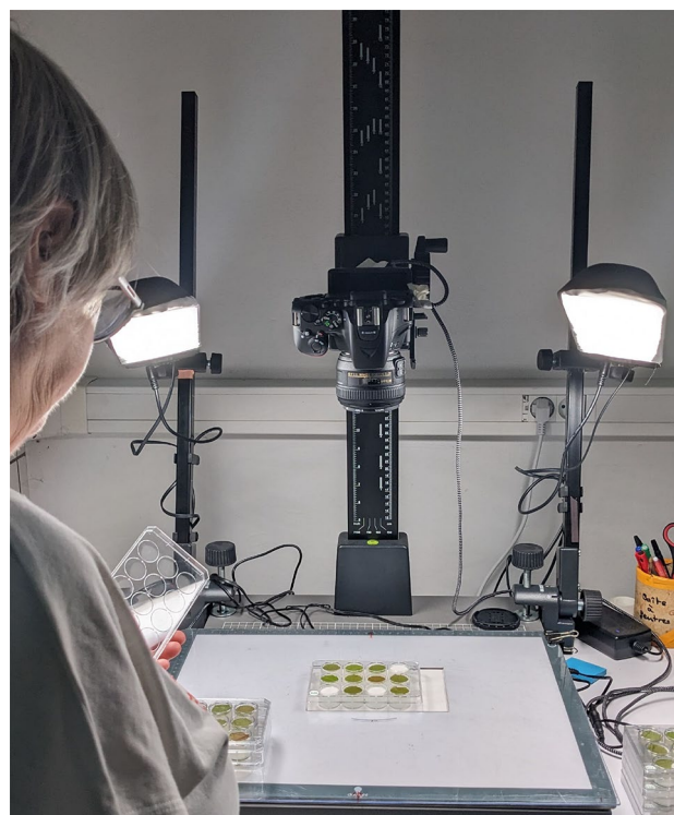
Fig. 3 Imaging system used to produce the original plate images
