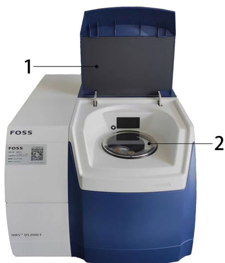
Fig. 2 FOSS NIR5™ DS2500F SR diffuse reflection near-infrared spectrometer (1 sample test bin covers 2 sample diffuse reflection test bin)
