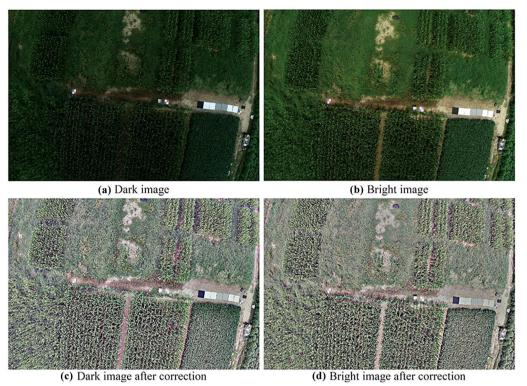
Fig. 7 The result of automated multi-scale Retinex correction. **a** The image collected under clouds shadow, and **b** the bright image was collected consecutively after the dark image when solar irradiance suddenly increased, **c** the illumination corrected dark image, and **d** the bright image after the illumination correction
