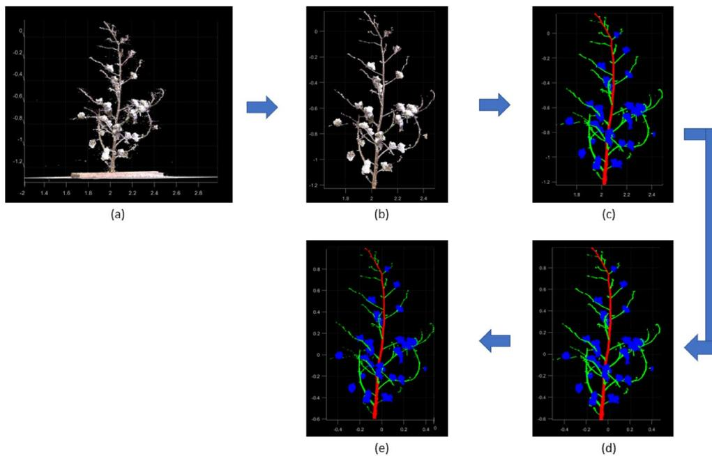
**Fig. 19** Data preprocessing steps on a sample input point cloud. **a** Input point cloud. **b** Denoised point cloud. **c** Labeled point cloud. **d** Normalized point cloud. **e** Down sampled point cloud
