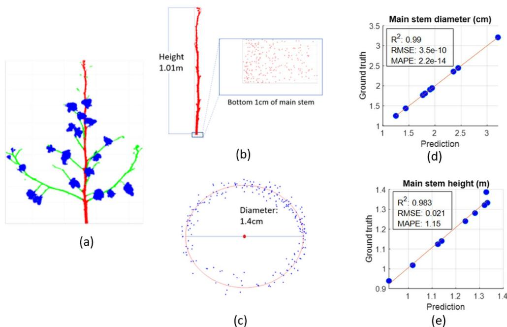
**Fig. 5** Main stem trait extraction and correlation with the ground truth. **a** Post processed sample from test set. The main stem, branch and bolls are segmented in red, green, and blue, respectively. **b** Main stem height estimation and selection of the bottom 1 cm region. **c** Circle fitting on points projected on the xy plane. **d, e** Correlation of main stem diameter and height extracted from predicted and ground truth segments
