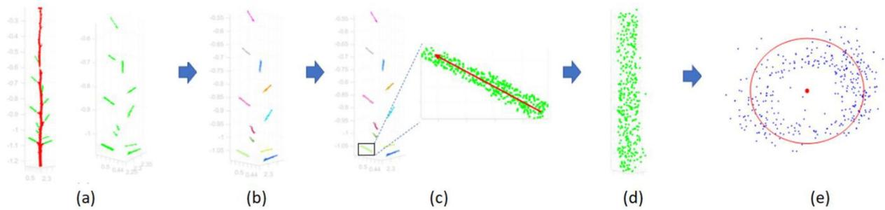
**Fig. 23** Branch traits extraction. **a** Segmented main stem and branch points within 6 cm from main stem. **b** Clustering of selected branch points. Each color represents a detected branch. **c** Principal component analysis applied on selected branch. Vector in red represents the principal component in the direction of branch **d** Vertical alignment of selected branch **e** Projection of points on xy plane and circle fitting
