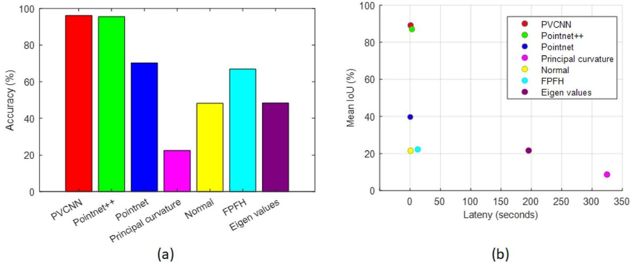
**Fig. 12** Comparison of hand-crafted features and the deep learning-based features for segmentation of main stems, branches and cotton bolls. **a** Segmentation accuracy **b** Time consumption (in seconds) vs mean IoU (%)
