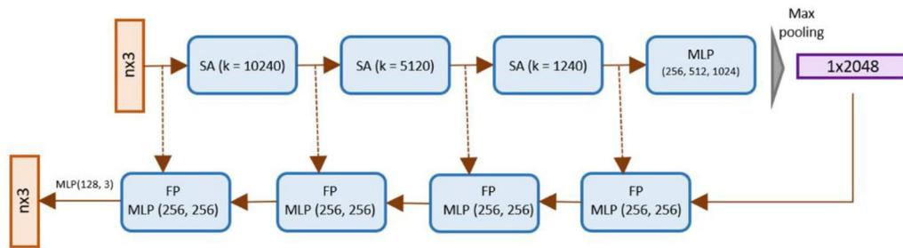
**Fig. 21** Pointnet++ architecture. Three set abstraction (SA) layers are applied and followed with MLP layer. The resulting features are aggregated using Max pooling and interpolated using four Feature propagation (FP) layers. The FP layers are followed by MLP layers and the final MLP layers are used to output scores per point
