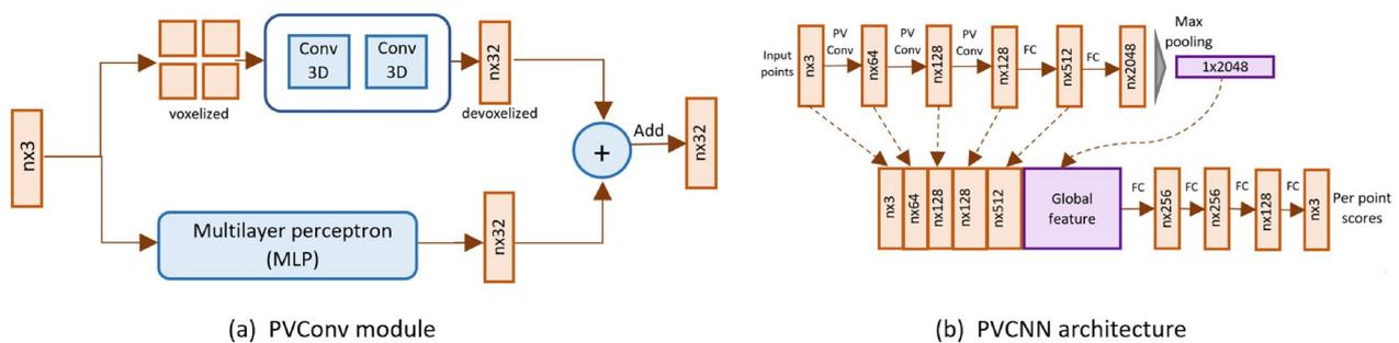
**Fig. 22** Point Voxel Convolutional Neural Network. **a** The PVCNN layer applies 3D Convolution on voxelized input. It devoxelizes the aggregated features back to map the points. The point-based and voxel-based features are fused to form the output. **b** The PVCNN network takes  $n$  points as input and applies PVCNN and FC layers. It then aggregates the point features by max pooling and concatenates the features to output scores per per point
