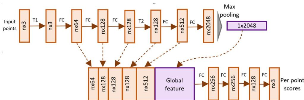
**Fig. 20** Pointnet architecture. The network takes  $n$  points as input, applies feature extraction. It then aggregates the point features by max pooling and concatenates the features to output scores per point. FC is fully connected layer operating on each point. T1 and T2 are transformation networks for input points and features
