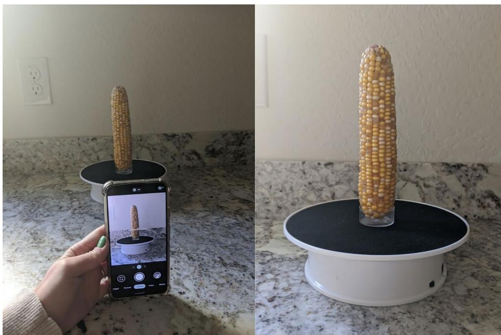
**Fig. 1** The Corn360 system. Panoramic image capturing as the corn ear revolves (L) and A corn ear is placed on the turntable (R). L left, R right
