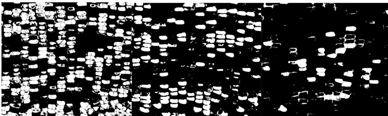
**Fig. 5** An example shows the Food Color Inspector segmented split channel adjusted binary images for the classes purple (L), white (M), and yellow (R) kernels of the mixed colored corn sample 1 shown in Fig. 4
