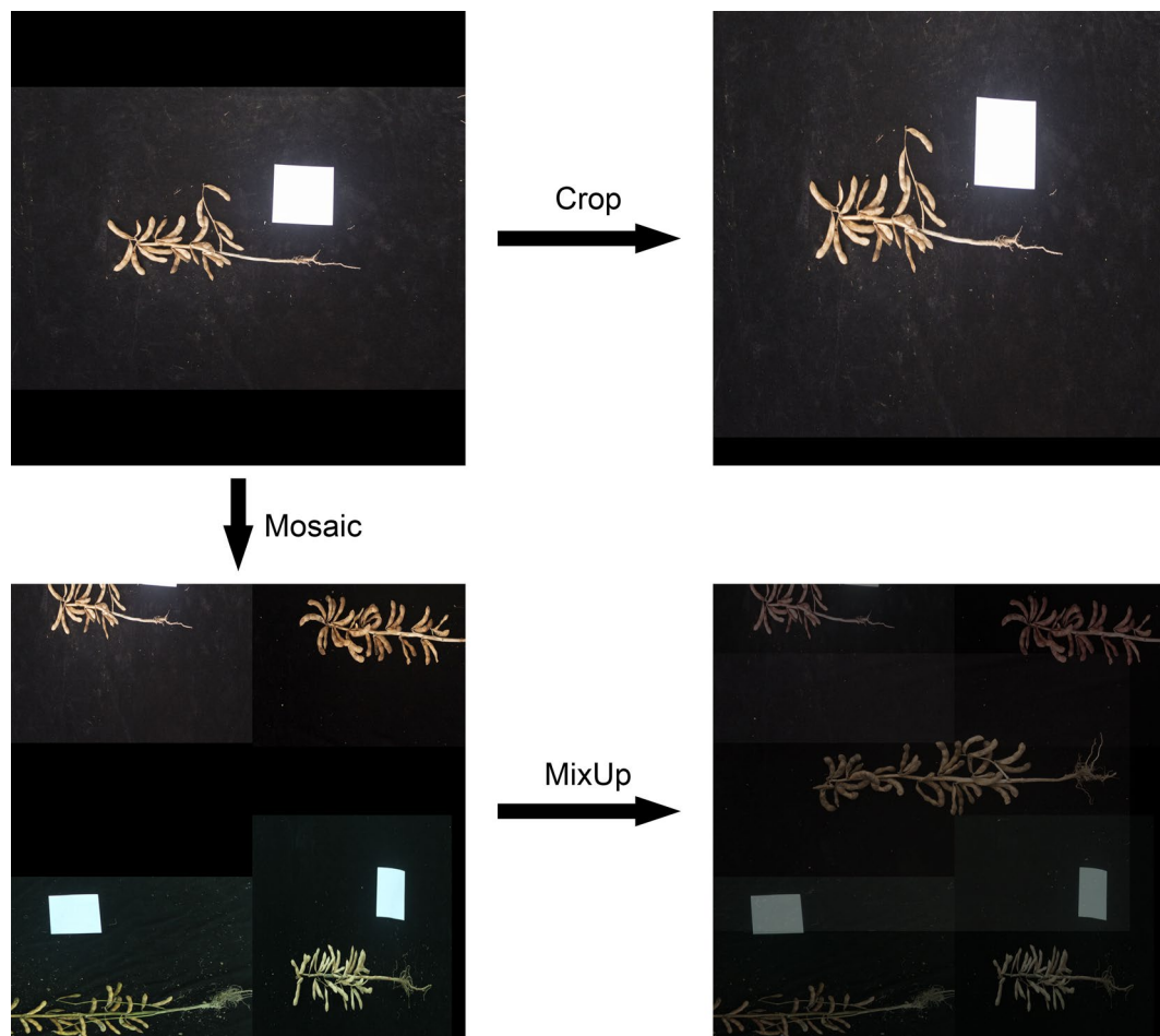
Fig. 2 Illustration of YOLO POD's image augmentation pipeline
