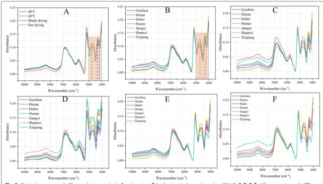
**Fig. 3** Original spectrum of different drying methods **A** and regions **B** for *E. ulmoides* leaves based on FT-NIR. **C**, **D**, **E**, **F**: different regions of  $40^{\circ}$ C,  $60^{\circ}$ C, sun drying, and shade drying, respectively
