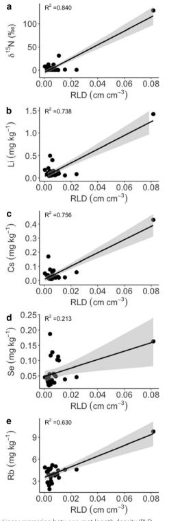
Fig. 9 Linear regression between root-length density (RLD; cm cm<sup>-3</sup>) and nutrient tracers (<sup>15</sup>N, Li, Cs, Se and Rb). The shaded area represents one SE
