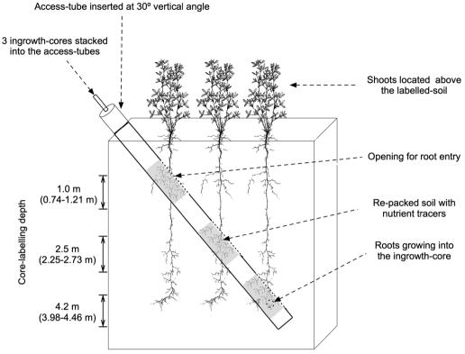
Fig. 3 A schematic diagram describing the concept of core-labelling technique (CLT); Figures of plants are from Kutschera et al. [31]
