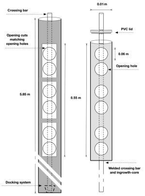
**Fig. 2** Schematic diagrams of an access-tube with ingrowth-core inserted (left) and an ingrowth-core (right)
