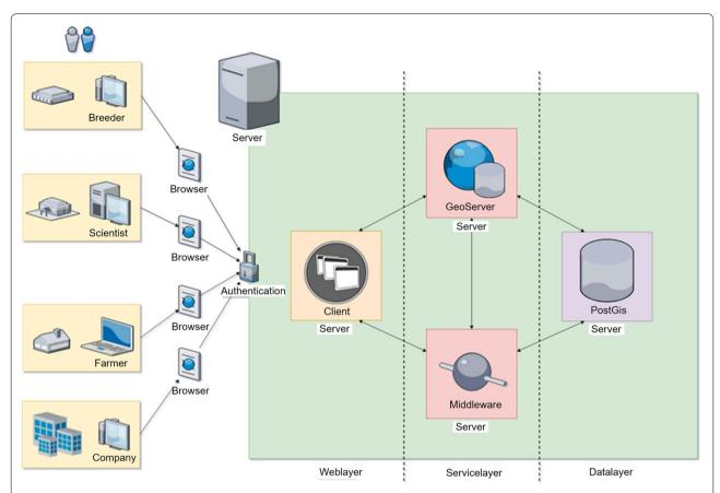
**Fig. 1** System architecture of the DMIS. Users authenticate and access the application on the server via browsers. The system components are installed in Dockers and communicate with each other via HTTP. The GUI (Client) is localized in the Weblayer, the PostgreSQL and PostGIS database components in the Datalayer, the GeoServer and a Middleware are acting in the Servicelayer, connecting the client application and the database
