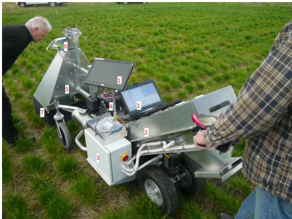
Fig. 1 The M5 Multi-Purpose Harvesting Imaging Vehicle developed and used to collect LiDAR data as described in this publication. 1: PC screens, 2: harvester, 3: control panel, 4: generator, 5: hood, 6: LiDAR scanner, 7: blackout curtain
