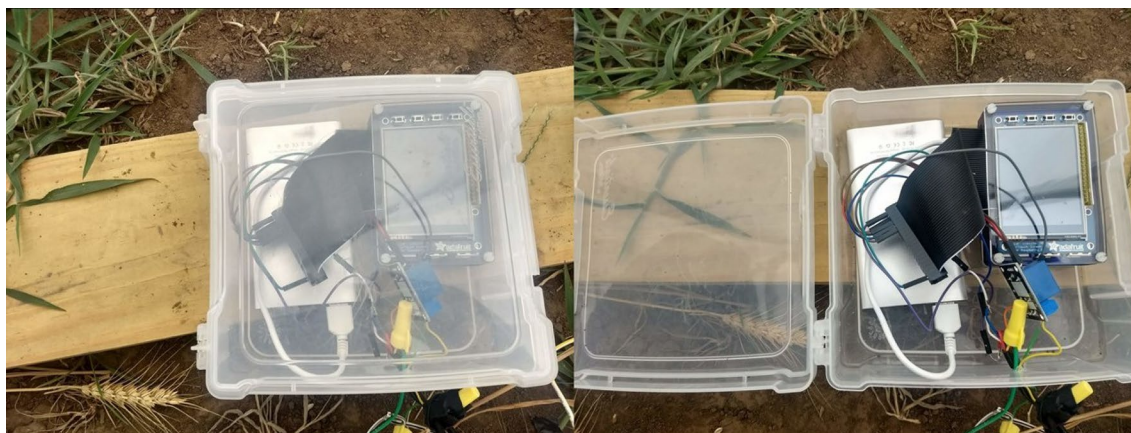
Fig. 3 Waterproof enclosure for Raspberry Pi and electrical system. The system was contained within a plastic box that latched closed (left) to protect the underlying circuitry and opened (right) to allow access to the system. Inside each enclosure was a battery pack, USB to microUSB cable to supply power, one Raspberry Pi computer with touchscreen display, a ribbon cable to extend connections to the computer, and a blue solid-state relay. A hole was drilled in the side of the enclosure to facilitate electrical connections to the heater circuit; this hole was filled with caulk for water protection
