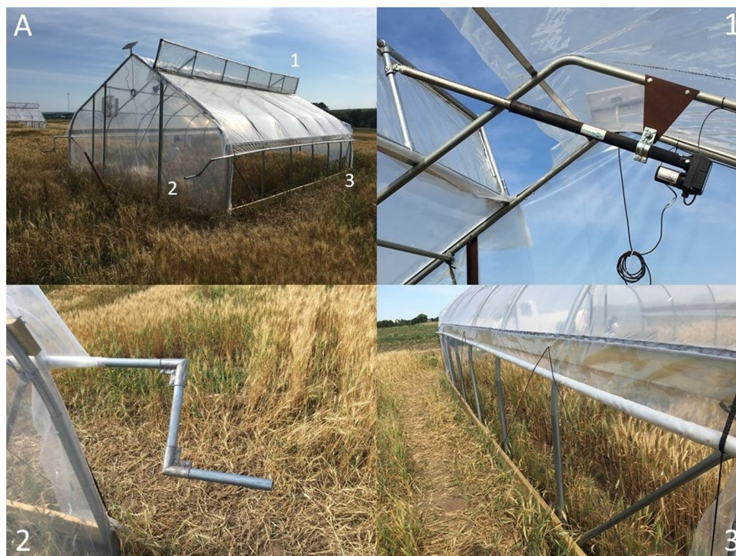
Fig. 1 Vent system layout. A HNT heat tent during daytime 1: venture manufacturing 12V linear actuator used to open top vent. 2: Handle used to manually operate side roll up ventilation. 3: Side rolled up with polypropylene rope securing it against the tent
