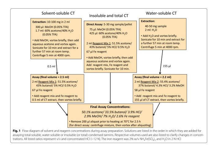
mixtures were centrifuged 5 min at 4000 rpm prior to taking non-heated and heated aliquots for absorbance readings, and pellets re-suspended by vortex mixing before heating.
