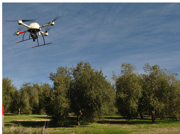
Fig. 10 The quadcopter UAV and the Red–Green–Blue (RGB) camera used to acquire the remote images of the olive trees
