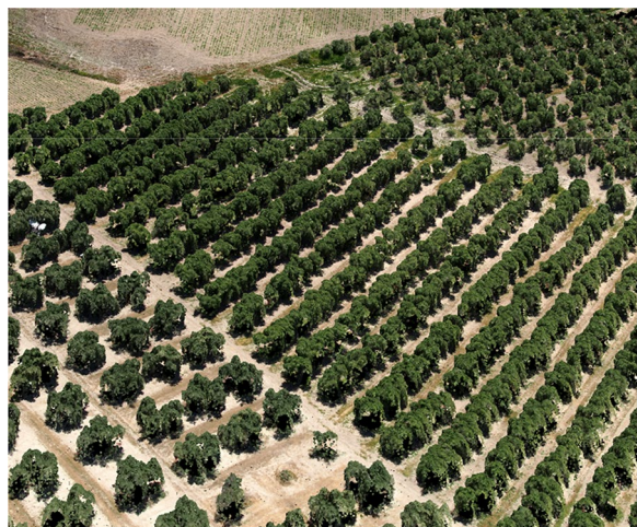
Fig. 11 A partial view of the 3-D Point Cloud for the olive grove studied in this investigation, which was produced by the photogrammetric processing of the remote images taken with the UAV
