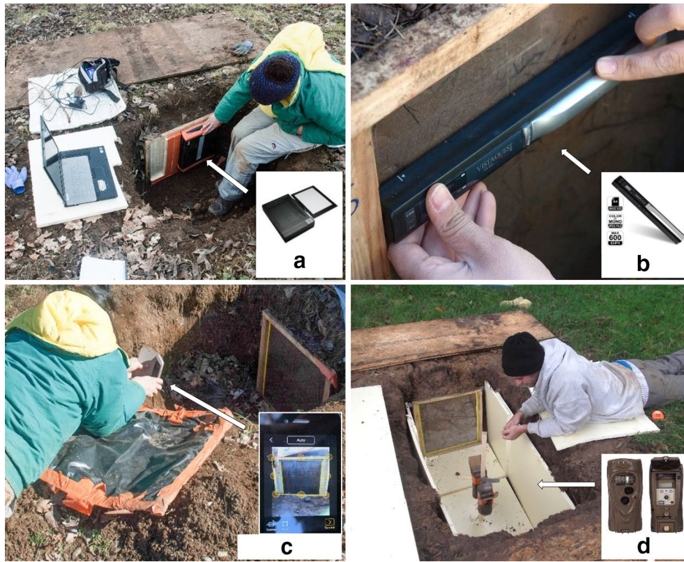
Fig. 1 Four different methods were used to take images of walnut tree roots in rhizotrons: a flatbed scanner, b handheld scanner, c smartphone scanning application and d time-lapse camera. In (d) , the time-lapse camera and rhizotron were placed into insulated boxes so that variations in temperature did not affect root growth. In the other rhizotrons, insulating material was placed over the rhizotron Plexiglas pane and removed before scanning
