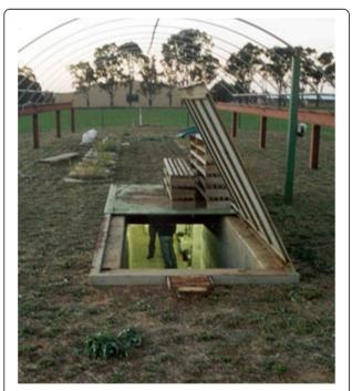
Figure 10 View of the surface and underground work area of the CSU rhizolysimeter complex. In the background, silos containing cores are growing lucerne, while in the foreground, the entrance and stairwell which provide access to the underground laboratory are visible.
