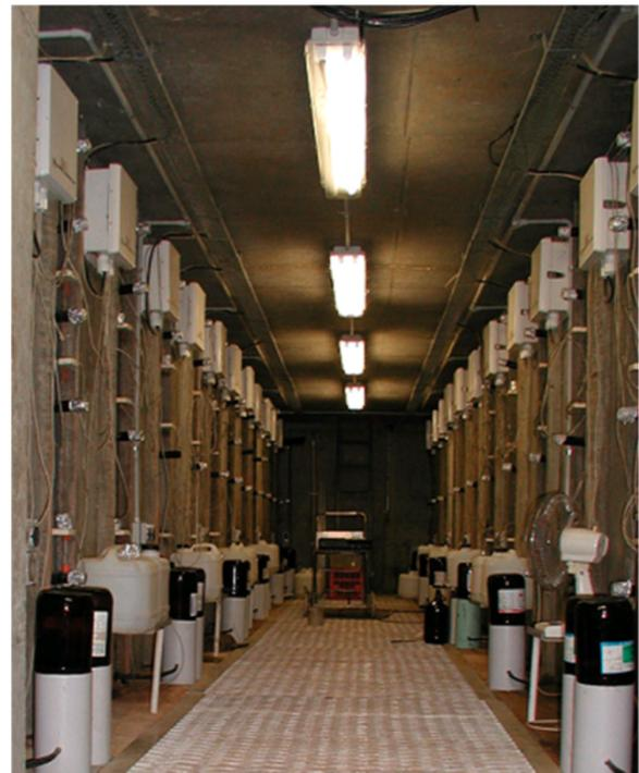
**Figure 11** The underground laboratory beneath the rhizolysimeter. The white boxes at the top of each core contain multiplexers and network the TDR signals emanating from each core. The black tubes covered with aluminium caps protruding from each core are exposed section of the mini-rhizotron root observation tubes.
