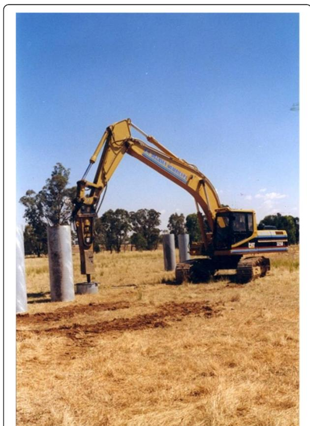
**Figure 14** Excavator hammering the steel core in to collect the undisturbed soil core.
