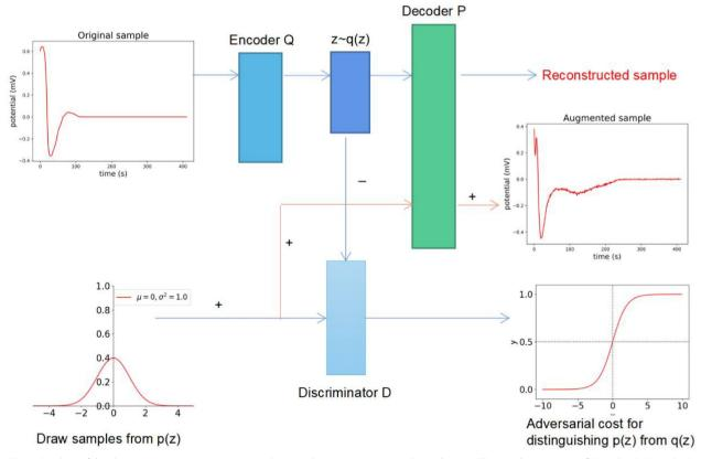
Fig. 3 Pipeline of the data augmentation.'+' represents the virtual vector,'' represents the real vector. The pipeline consists of Encoder Q, Decoder P and Discriminator D. The curve in the lower left corner is a Gaussian distribution plot. The curve in the lower right corner shows a sigmoid function
