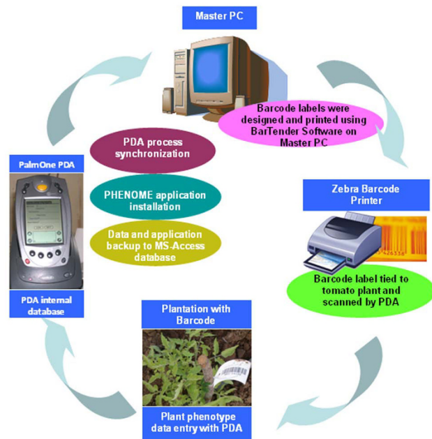
Figure 1 The cycle of plant phenotype data collection using PDA with PHENOME software. Plant ID barcode labels are tagged to plants. Using PDA phenotype data of plant is collected in the internal database of PDA. Once the PDA is synchronized with Master PC, the data from PDA database is synchronized with MS-Access database. The process to collect and synchronize the plant phenotype data using PDA from the field is cyclic process. For further changes in the plant phenotype catalogue, the modification has to be done in PHENOME software and it needs compilation and synchronization with PDA to update the changes (The process of modification in the PHENOME software is given in "PHENOME Read Me" file).
